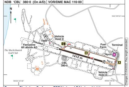
Surface Rwy Dim(m) TORA(m) LDA(m) Lighting 11/29 † Thr Rwy APAPI 3° 1412x46 Concrete/ 11-1412 11-1412 † Thr Rwy APAPI 3.5° Asphalt 29-1412 29-1412 † Thr and Rwy portable electric during night hours only.
