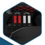
The base includes a switch panel with master, avionics and light switches as well as red LED backlighting for night operations.
