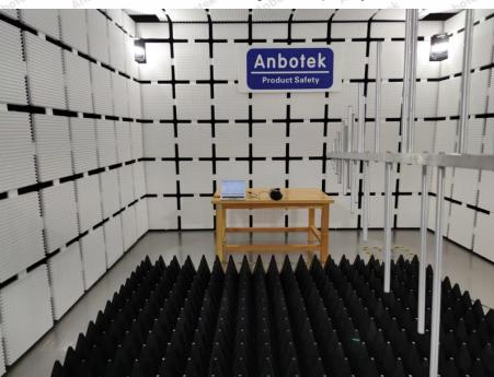
Photo of RF Field Strength susceptibility Test
