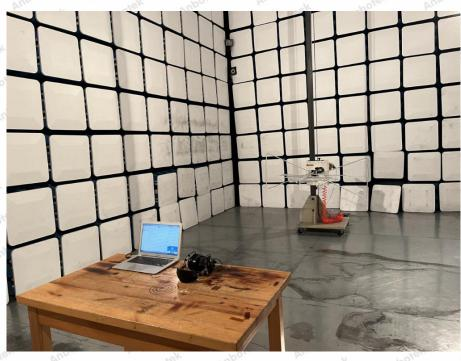
Photo of Electrostatic Discharge Immunity Test
