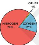
A given volume of pure, dry air contains about 78% nitrogen, 21% oxygen, and a 1% mixture of 11 other gases. Air also can contain water vapor, which varies from 0 to 5% by volume and takes the place of an equal volume of dry air.
