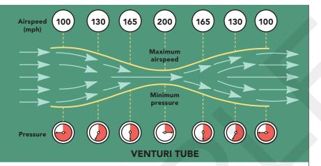
**AIRSPEED AND AIR PRESSURE** are related in a way that is crucial to flight. This relationship is illustrated by the flow of air through a *Venturi tube*. As air flows through the constricted throat at the center of the tube, it speeds up in the same way that water does when it flows through the nozzle of a garden hose. As the air leaves the constricted throat of the Venturi tube, its speed decreases.
