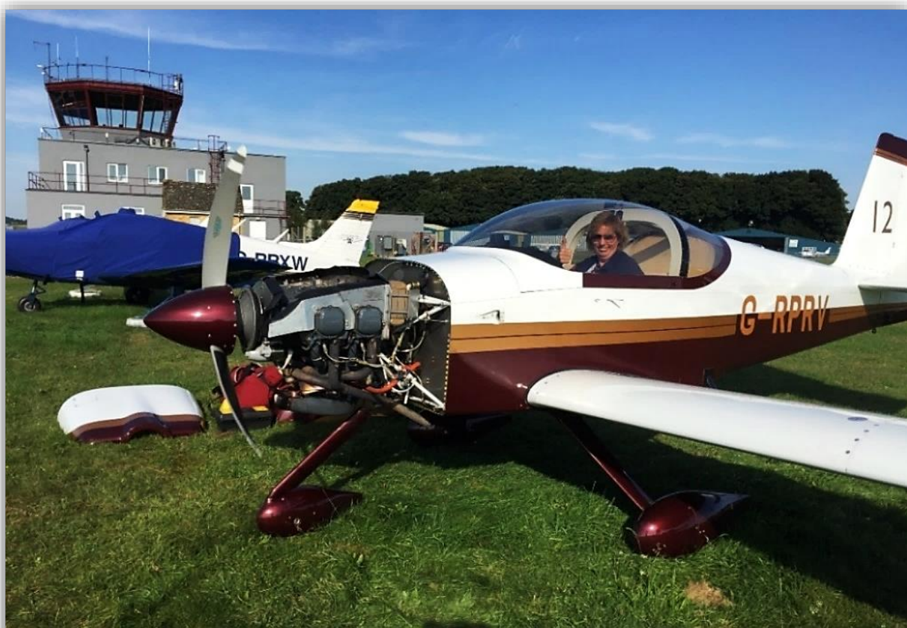
Cowling off, full inspection of engine: a loose contact to the battery was found
