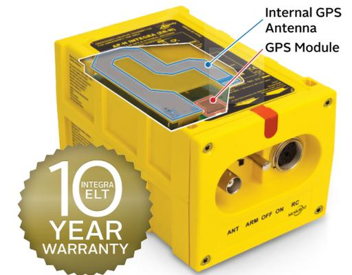
The Kannad Integra ELT offers additional safety benefits including automatic activation through an internal G-Switch and a 406 back antenna offering the highest level of resiliency.
