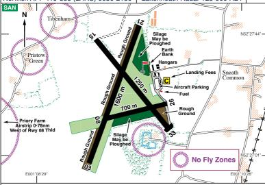
Surface TORA(m) LDA(m) Lighting Rwy Dim(m) 03/21 1600x46 Asphalt Unlicensed Nil 08/26 700x46 Asphalt Unlicensed Nil 15/33 1250x46 Asphalt Unlicensed Nil
